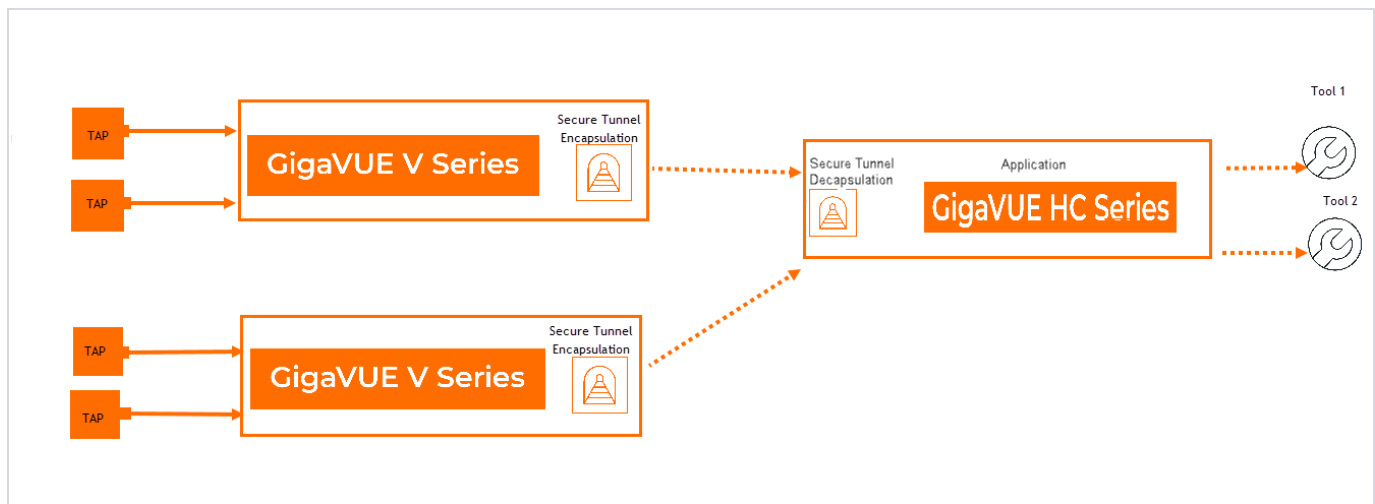
Figure 104 GigaVUE HC Series with a single IP Interface and multiple Map rules
