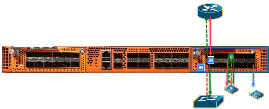
Figure 52 Logical Bypass Without Bypass Combo Module
