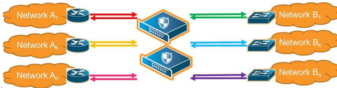
Figure 26 Inline Tool Inserted in Multiple NetA-NetB Links
